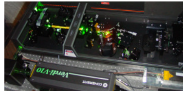
Pump laser (green), Ti:Sa laser (red) and 2HG (blue)
