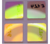
dielectric Bragg mirrors from MgO/ZnO 2
