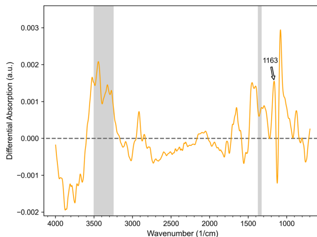
Fig. 4 Differential FT-IR spectrum of SMXder functionalized PEG hydrogel microparticles. The FT-IR signals of neat, unfunctionalized particles and SMXder functionalized particles were annealed via the classical least squares method before subtracting the former from the latter. The typical vibration signals of sulfamethoxazole are shaded in grey between 3500 \text{cm}^{-1} to 3250 \text{cm}^{-1} and 1370–1330 \text{cm}^{-1} as well as annotated at 1163 \text{cm}^{-1} .
