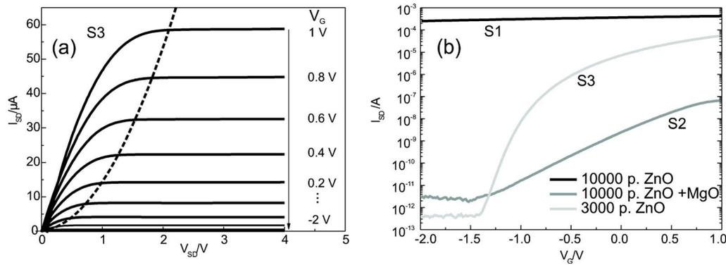
FIG. 3. (Color online) (a) Source-drain  $I$ - $V$  output characteristic of sample 3 for different gate voltages. The dashed line is a quadratic fit of the pinch-off points. (b) Transfer characteristics of samples 1, 2, and 3. (Note that sample 1 is not in saturation regime.)
