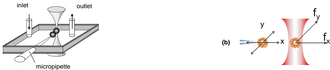
Fig. 1 Scheme (a) of the sample cell to measure forces between two separated colloids and scheme (b) of the direction of motion
