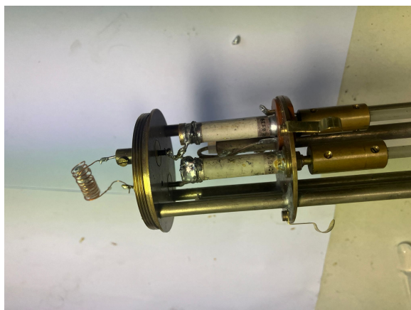
Figure 4: Inside the probe: a coil sits at the end, enclosing the sample. The two legs are connected to the hotwire and ground, respectively, while the white cylinders are adjustable capacitors.
