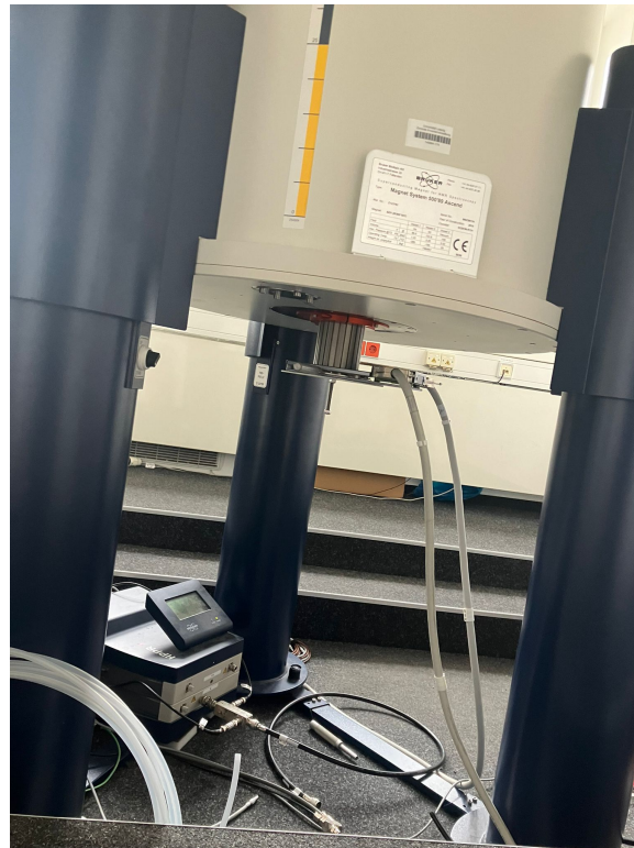
Figure 3: View inside the lab: A 500 MHz magnet. The inserted probehead can be seen at the bottom.
